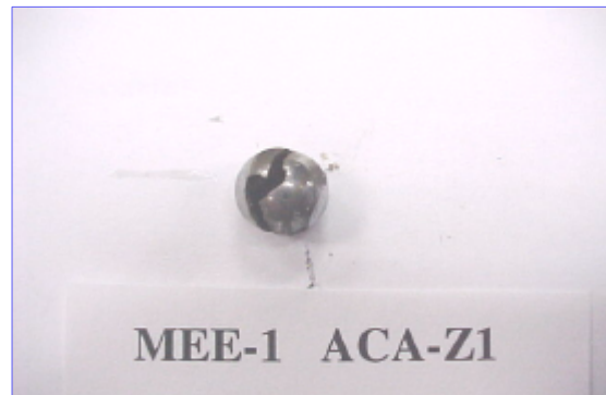
Figure 18: Cleaved Diverter Ball from MEE-1 Test
